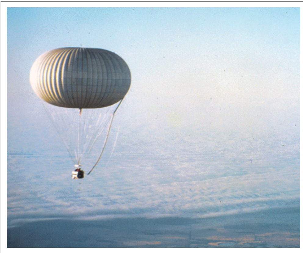
Fig. 7. Example of a 15-m-diameter high-altitude helium balloon, operated at 0.1 atmosphere pressure, during Nott's 1984 crossing of Australia.
