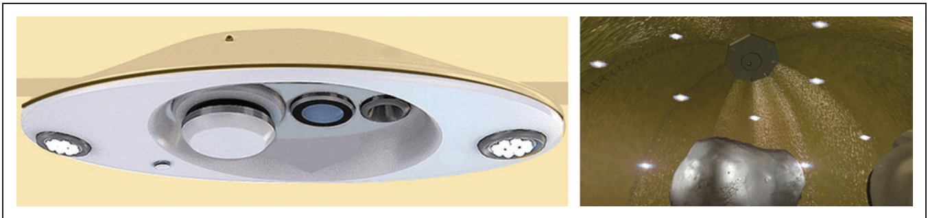
Fig. 5. Detail of camera unit with (from left to right) lights, pressure/temperature sensors, vent to envelope, camera, and gas thruster. The thruster is mounted on a high-pressure supply gas line, while a data and power line connects computer with camera, lights, thruster, and vent.
